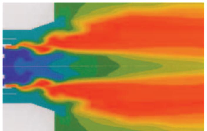
CFD Modelling of a Low NOx Burner (courtesy Mitsui Babcock Energy Ltd)
