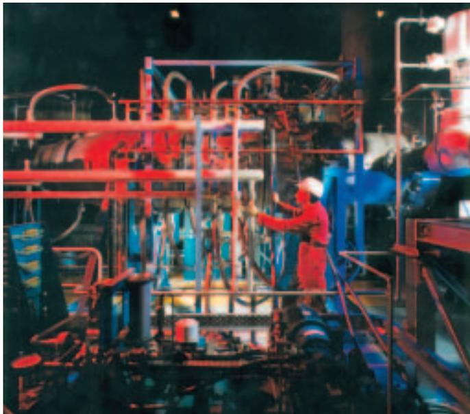
High Pressure Gas Turbine Combustion Rig (courtesy ALSTOM Power)
