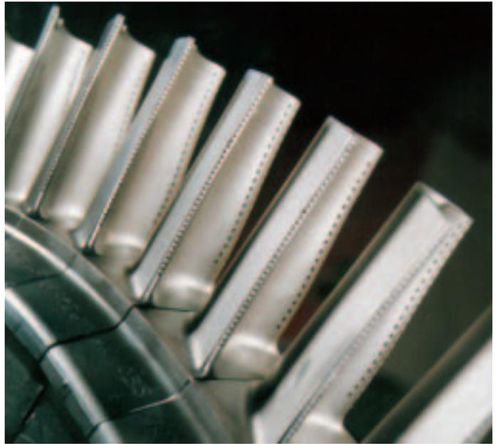
Cooled Turbine Blades (courtesy ALSTOM Power)
